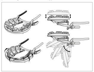
Self-adjusting petals flex and pivot to adapt to the unique shape of your client's face, providing ultimate client comfort
